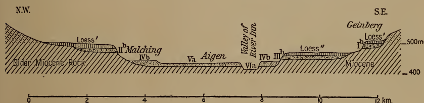
FIG. 6. Terraces on either side of the valley of the River Inn, Scharding, Austria, formed by sand and gravel deposits partly covered with loess. After Brückner.
