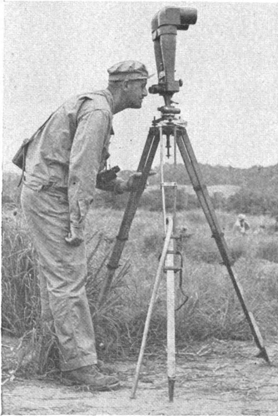
Figure 300. Battery commander's telescope. Although giving a high magnification and wide field of view, the individual telescopes cannot be placed in a horizontal position to improve stereoscopic vision.
