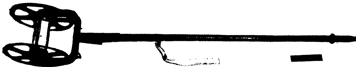
Figure 371. Hand wire reel unit with broomstick handle.
