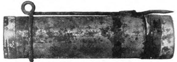
Figure 276. Self projecting vomiting gas candle.
