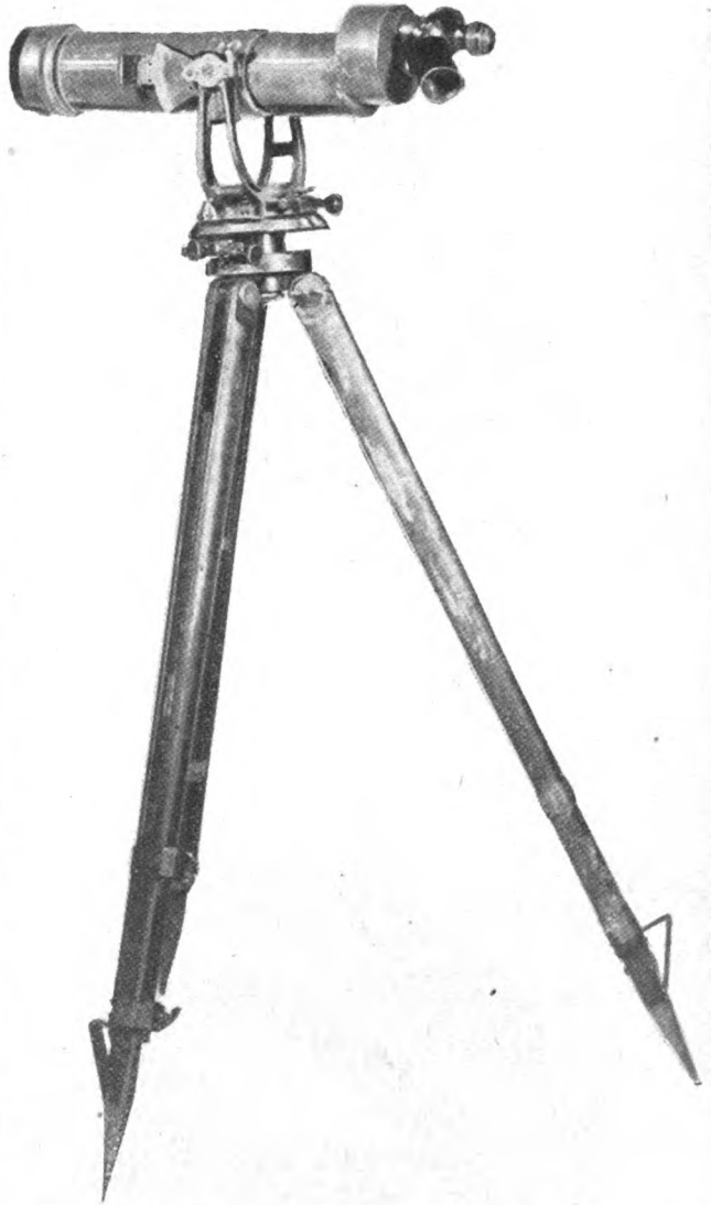
Figure 301. This artillery spotting telescope may be used with three different eyepieces, each of which gives a different magnification—the maximum being 33 power. Provision is made to measure azimuth, and elevation (from -30^{\circ} to +30^{\circ} ).
