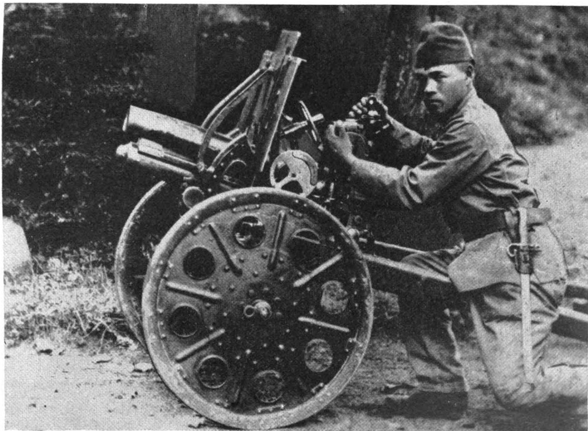
Figure 214. Photograph of model 92 (1932) 70-mm howitzer (Bn. gun) showing gunner and sights.
