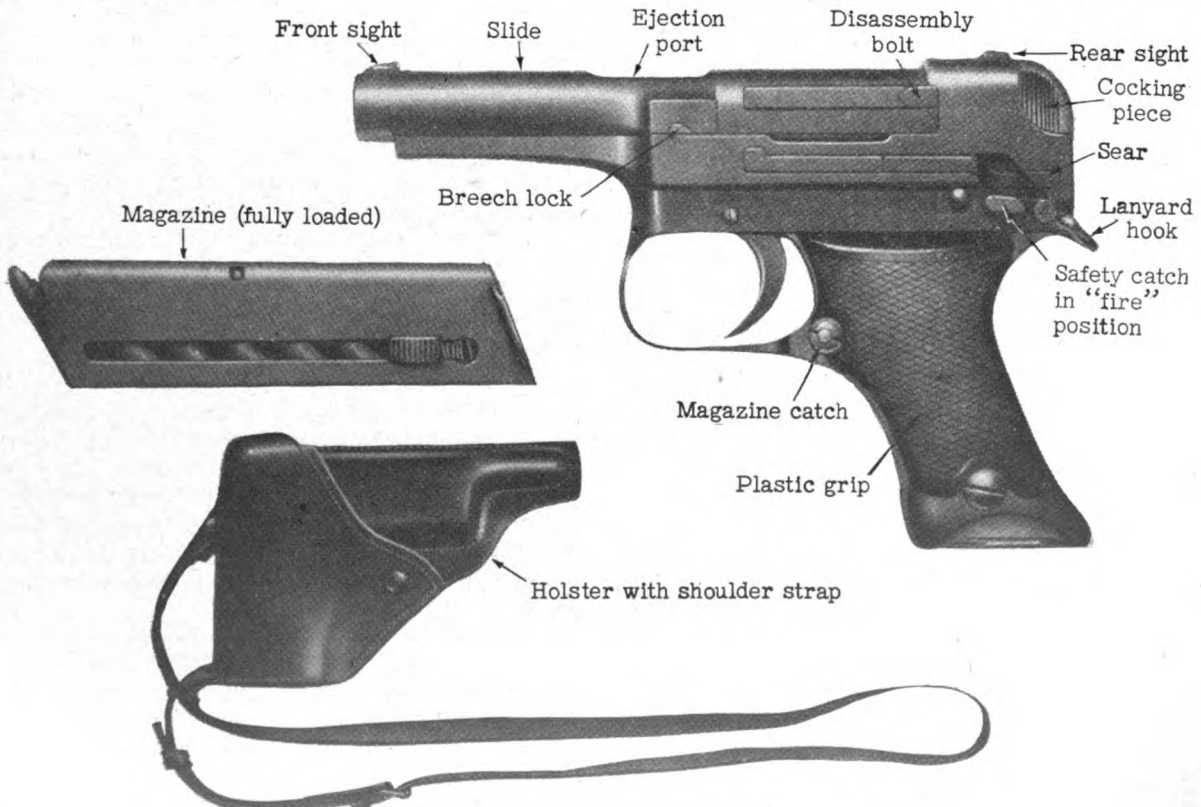
Figure 169. Model 94 (1934) 8-mm pistol, showing holster and magazine.
