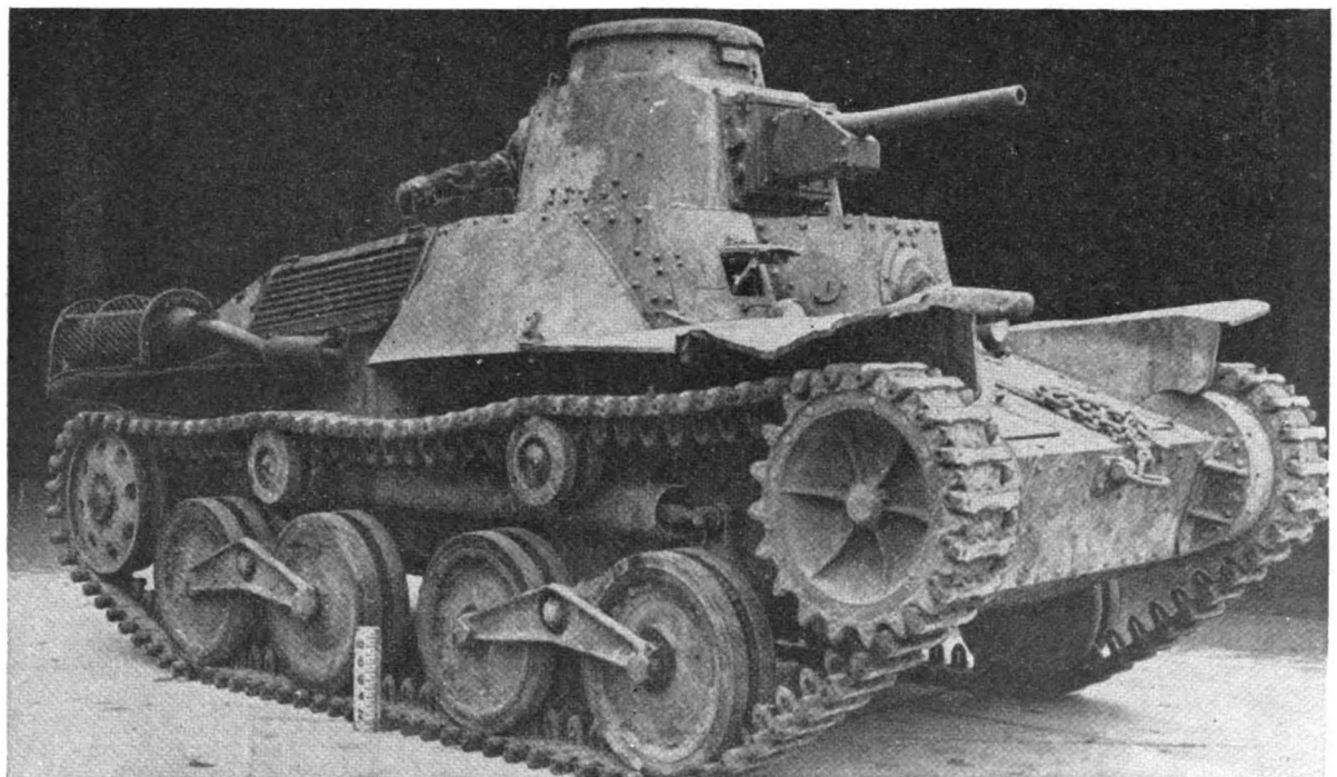
Figure 244. Model 95 (1935) light tank.
