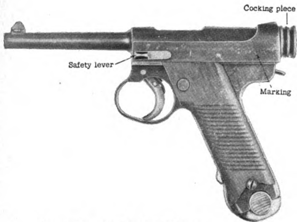
Figure 168. Model 14 (1925) 8-mm pistol.
