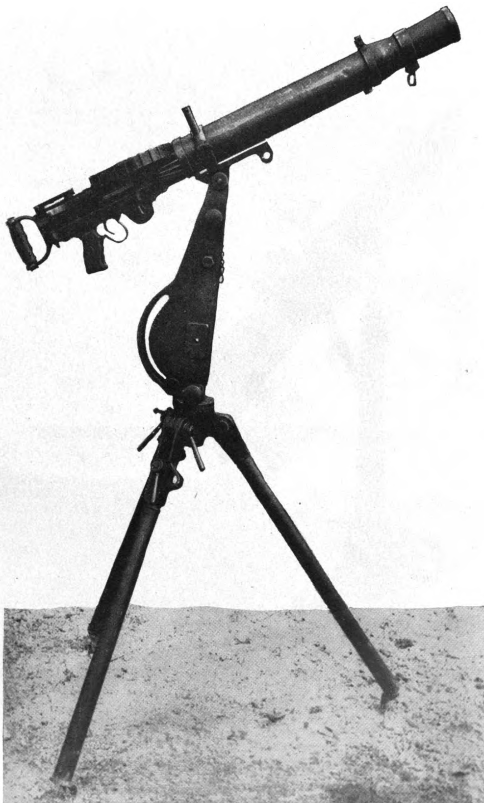
Figure 230. Model 92 (1932) 7.7-mm machine gun (Lewis type) in position for AA fire.
