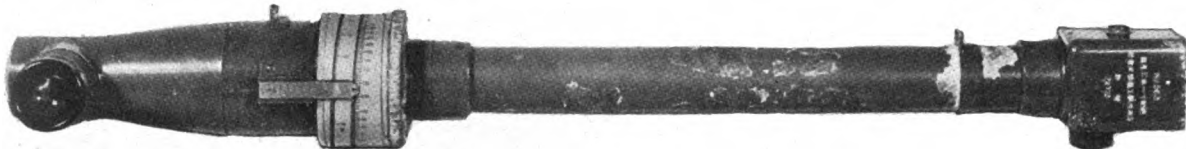
Figure 286. Model 92 (1932) 40-cm base range finder is calibrated for measuring ranges up to 1,500 meters (1,640 yards). It is a coincidence type of range finder with a 4 × magnification.
