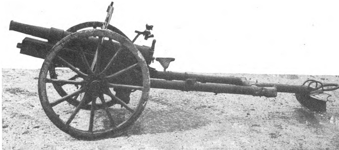
Figure 215. Side view of model 41 (1908) 75-mm infantry gun, showing unusual trail construction.
