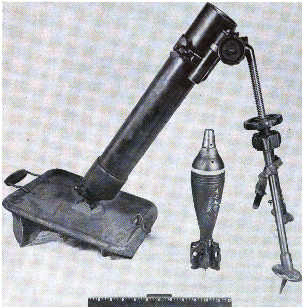
Figure 192. Model 99 (1939) 81-mm mortar and standard projectile.
