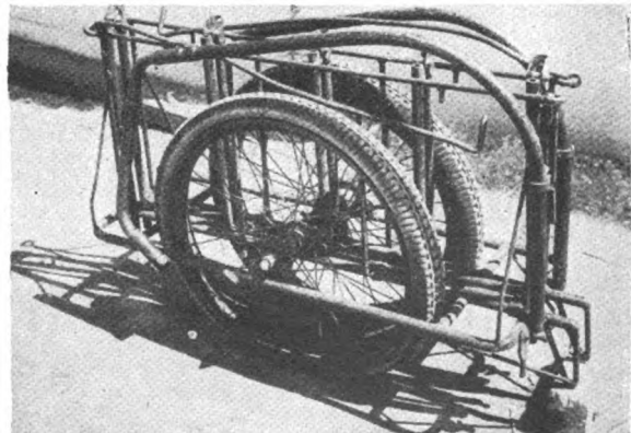
Figure 405. Collapsible hand cart of metal construction weighing 100 pounds. It may be pulled by hand or towed by bicycle.
