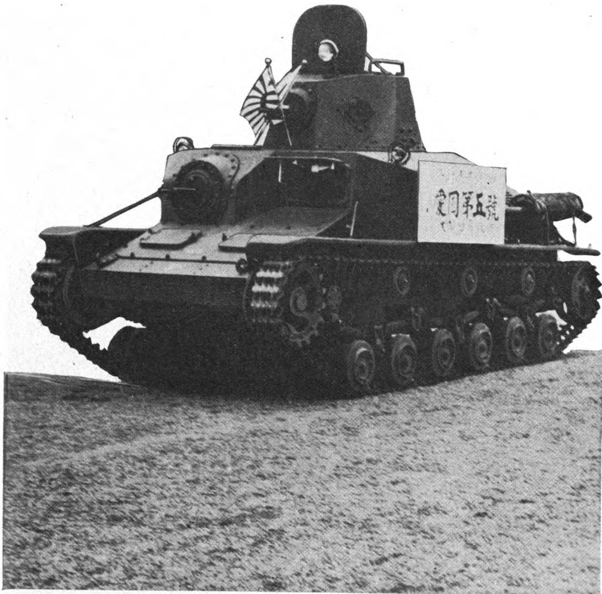
Figure 243. Model 93 (1933) light tank.
