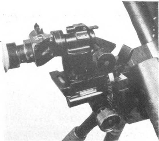
Figure 288. Panoramic sight for model 94 (1934) mortar has a 3 × magnification and a 13° field of view. Micrometer drums enable readings to be made to the nearest mil.
