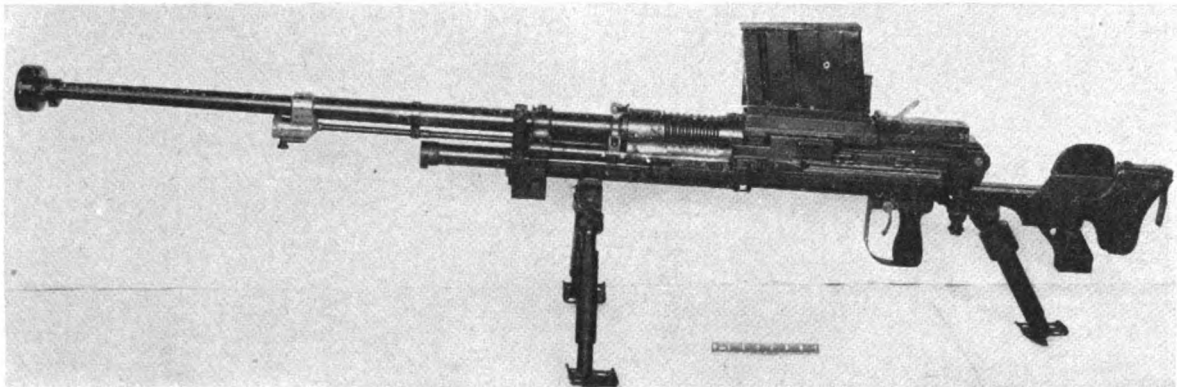
Figure 209. Model 97 (1937) 20-mm antitank rifle.
