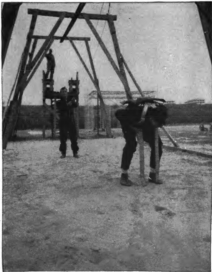
FIGURE 28. —Landing trainer. Instructor pulls release mechanism, allowing student to drop to ground.
