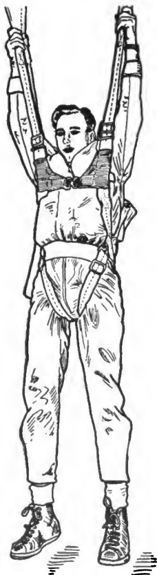
FIGURE 21.—Suspended harness training showing method of grasping risers.
