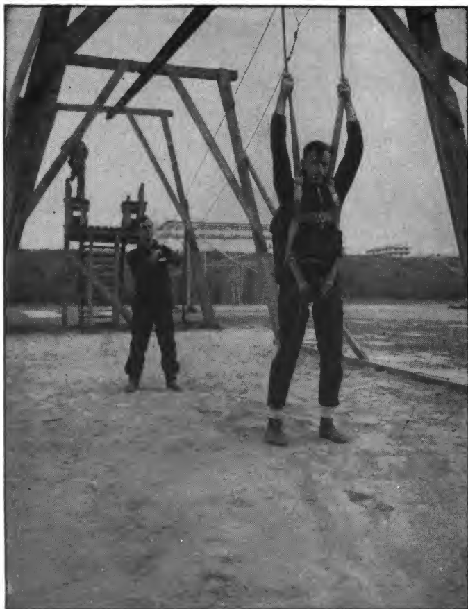
FIGURE 27. —Landing trainer. Student's feet touch ground momentarily at lowest position of inclined beam.
